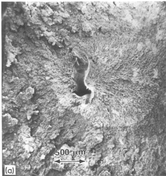
Figure 8 (a) Typical tensile fracture surface in the HI-POM core. Note the penny-shaped macrocrack which initiated brittle behaviour in the core. (b) Demarcation between (bottom) the drawn material within the macrocrack and (top) the plate-like fast-fracture region in the core of the HI-POM material.
